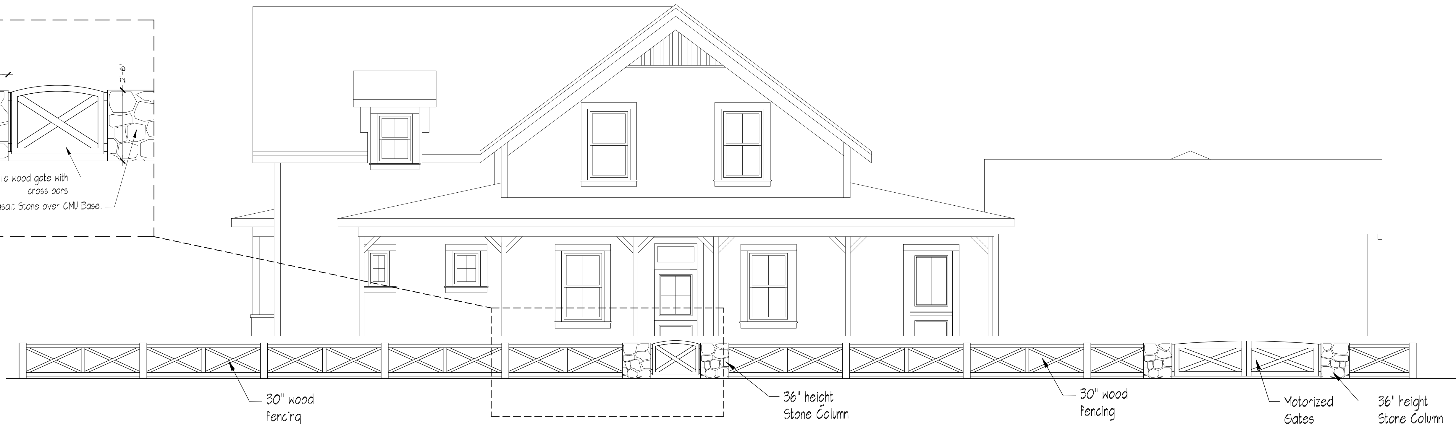
Jefferson Street Fence Elevation SCALE: 1/4" = 1'-0"
